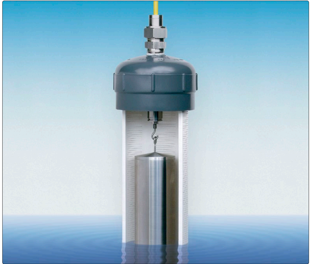
• The Model 4675LV with cutaway revealing its internal components: a cylindrical weight suspended from the vibrating wire force transducer.
